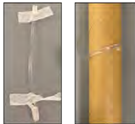
Figure 2: Photographs of contrast-filled nasal cannula in straight (left) and curved (right) configuration on CT gantry
