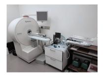
the-art Tera-TomoTM 3D PET image reconstruction engine. High imaging throughput can be obtained by large bore size and large field-of-view in both axial and transaxial directions in addition to multiCell imaging chambers for mice, rats and rabbits and a PrepaCell Preparation station
